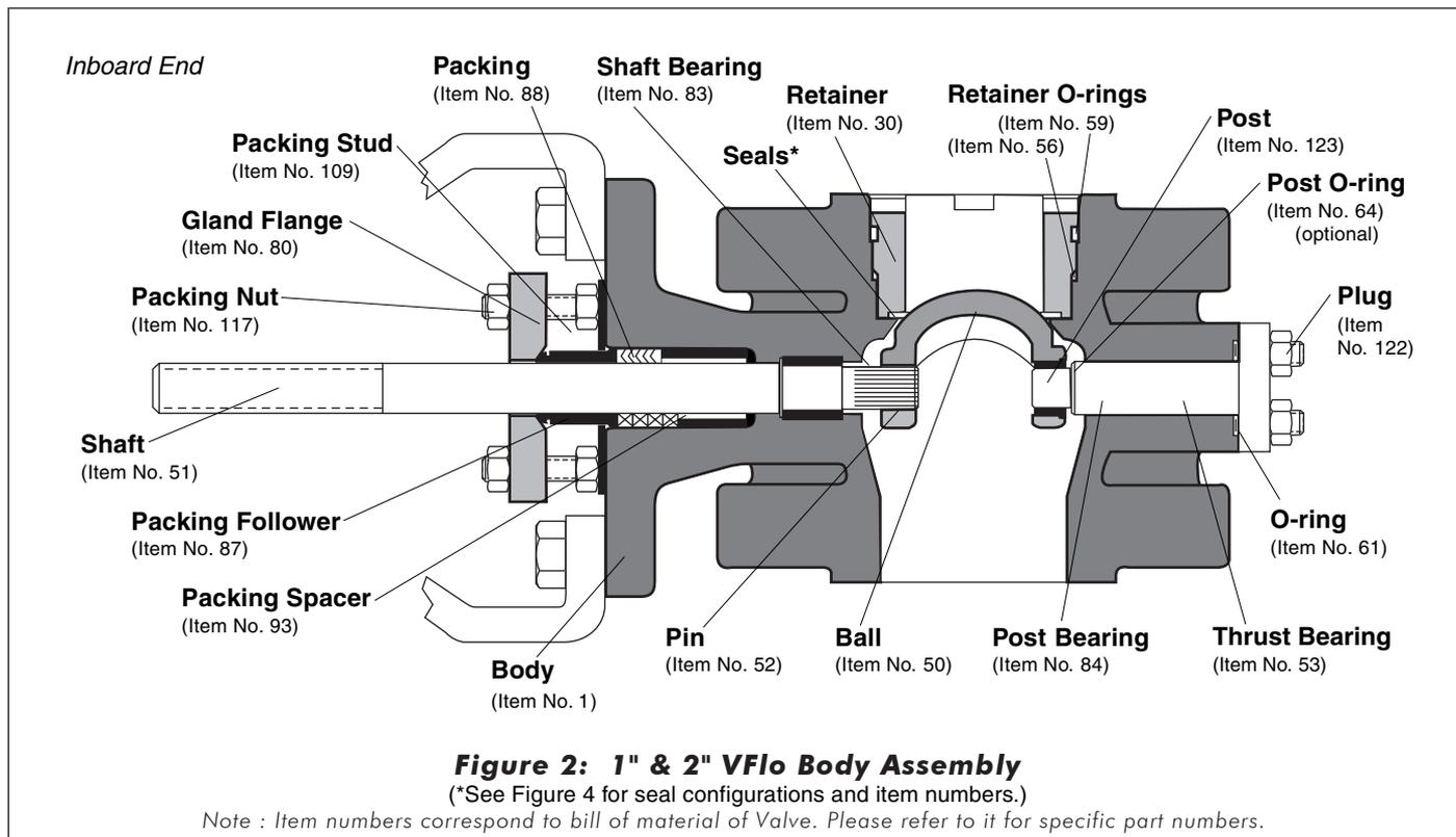
5. Rotate the ball inside the body in a way so that the non-splined end of the ball is toward the back port of the valve. Remove the ball straight out of the body. If needed, on stationary post designs remove the post bearing from the ball by pushing it out with a press.
