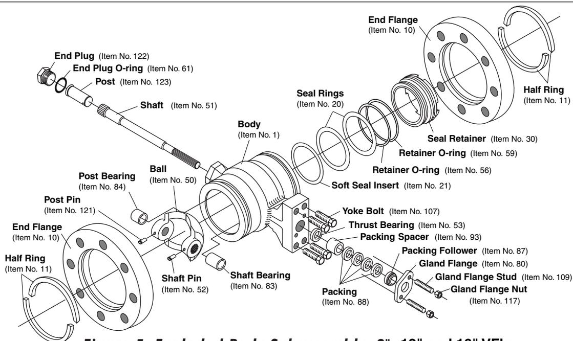
Figure 5: Exploded Body Subassembly, 3", 12" and 16" VFlo
